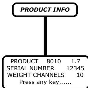
This page is purely for information purposes only. It shows the product name, BW8010, the software version, 1.7, the serial number, 12345 and the number of channels that are being used. Once any key is pressed the unit will return back to the Factory Set-up menu.
